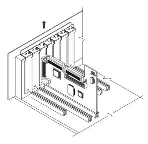
Figure 1-4. Host Bus Adapter Installed in 64-bit Slot
